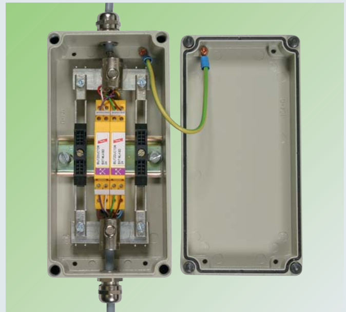
Lightning current carrying DIN rail mounted shield connection system, ideally suited for small cables. Slipping spring element compensates the yield of the cable materials.
