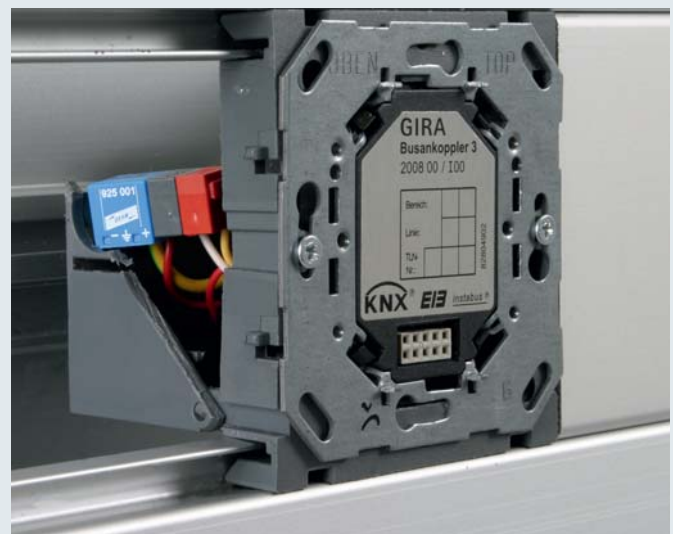
Protection of a KNX bus coupling unit by means of a BUSector surge arrester mounted on a bus terminal in the mounting panel of a cable duct.
