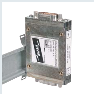
USD surge arresters are snapped onto a DIN rail. Overvoltage is discharged via the DIN rail.
