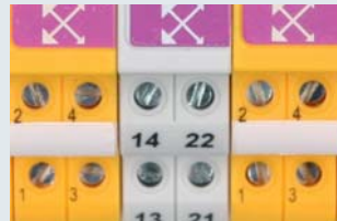
Floating remote signalling contact DRC MCM XT: break contact (21/22), make contact (13/14) DRC SCM XT: break contact (21/22)
