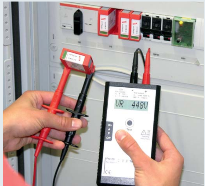
For testing the sparkover voltage of surge arresters. The specimen is connected via the included test leads or special test adapters.
