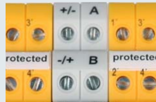
RS485 communications interface A/B (only for DRC MCM XT).
