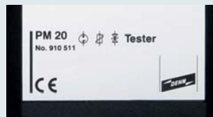
The response characteristics of gas discharge tubes, varistors and Zener diodes can be tested.
