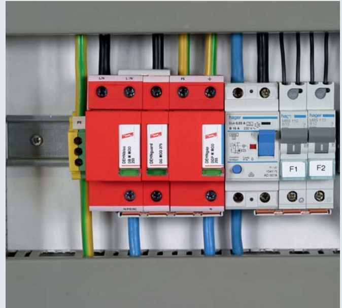
For protecting low-voltage consumer's installations against surges and even direct lightning strikes. For installation in conformity with the lightning protection zone concept at the boundaries from 0_A - 1 (3+1 circuit).
